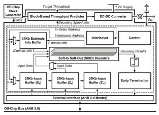
Fig. 3. The system architecture.
