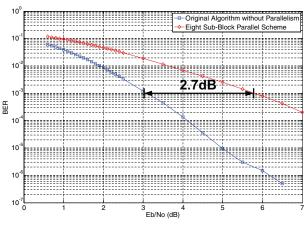
Fig. 1. The BER performance comparison between the algorithm [7] implemented without parallelism and with the eight sub-block parallel decoding scheme [3]–[5] when the block size is 40.
